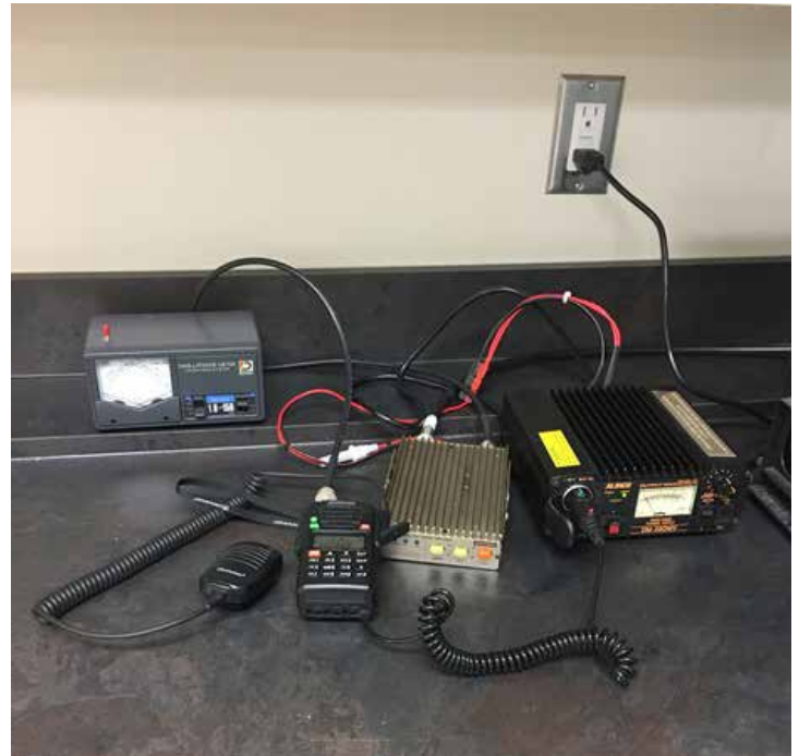
Photo showing power supply, 2 meter hand held radio and cable connection
