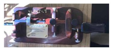
This bug was hand built by NA6O Gary Johnson. The tensions are magnetic and the dit contact is a magnetic switch.
